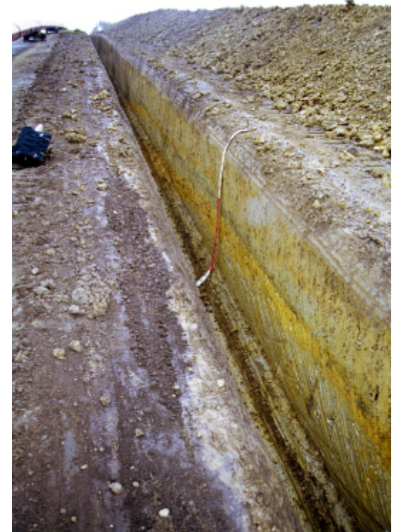
Slip plane features evident in trench below SW53: view downslope (left) profile view (centre), view upslope (right)
